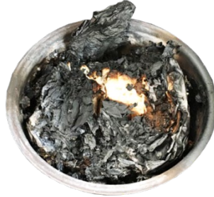
Residual waste due to bad incineration.
