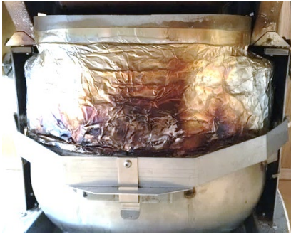
Residual waste due to bad incineration.
